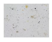
With filtration NAS 11 (12 mg/l) Varnish, metals, silica particles
