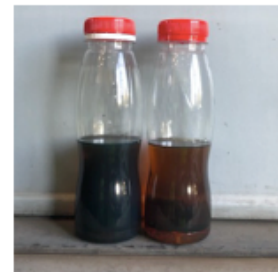
HYDRAULIC OIL BEFORE FILTRATION AND AFTER
