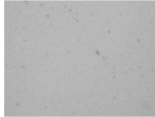
WITH FILTRATION 12485 HOURS 25.03.2018 NAS 7
